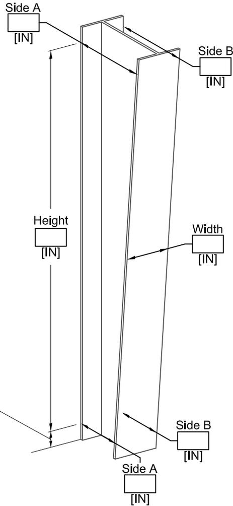
4" MAXIMUM ALLOWABLE DIMENSION TO MINIMIZE THE POSSIBILITY OF BODY CONTACT WITH THE WALL (Per ASTM Standard Specification F2440)
