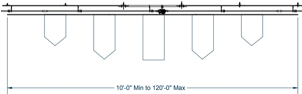
Banners Attach to 1 5/8" Suspended Tube. Tube supported a minimum of every 15' by 1/8" Cable supported in Cable Drums. Banners may need to be positioned or altered to attach.
