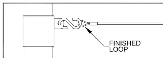
8. Feed the unfinished end over and through the pulley, finish attaching the net using instructions provided in the net box.
