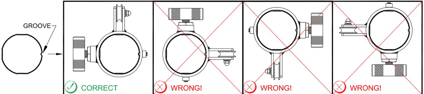
3. Adjust the spring plunger with a slotted screwdriver so that ball tip almost bottoms out in groove on upright. Do not adjust the spring plunger too tight against the upright, as it may be difficult to slide the sleeve up and down for net height adjustment. Tighten pressure lock assembly slightly to prevent sliding of the sleeve.
