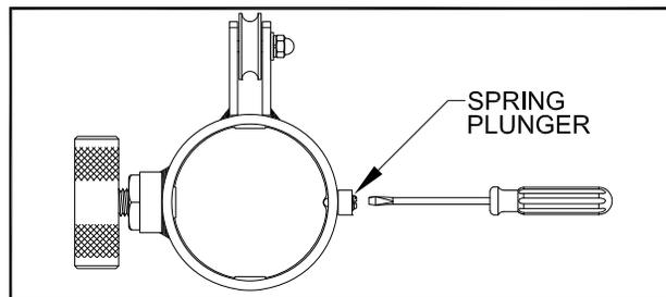
4. Assemble sleeve with net tie-off onto other upright assembly in the same manner as the sleeve with pulley in Step 2. Upright has 3 flat sides and 1 grooved side, be sure that ball tip on the spring plunger is riding in the groove on upright.
