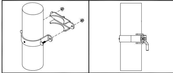
3. Attach winch using instructions provided in the winch box. Winch will attach over top of the tie-off assembly.
