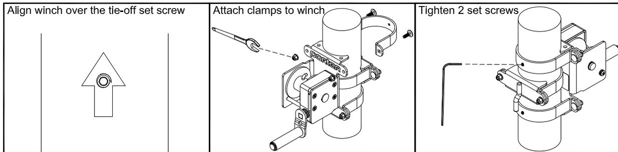
4. Place assembled standards in floor sleeves. Rotate standard until winch and tie-off are oriented as shown in the detail on Page 1.
