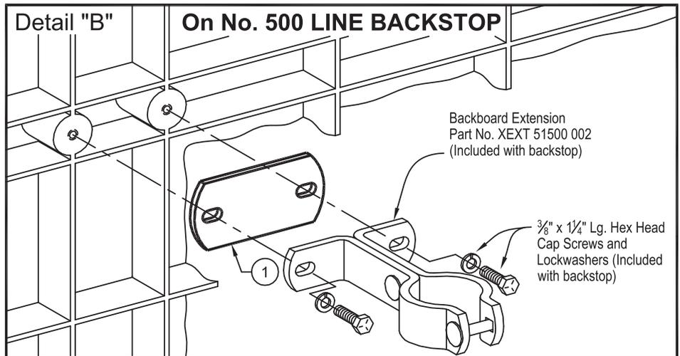
See opposite side of this page for instructions on installing a No. 216 Fiberglass Backboard on a ceiling-suspended backstop With a height adjuster.
