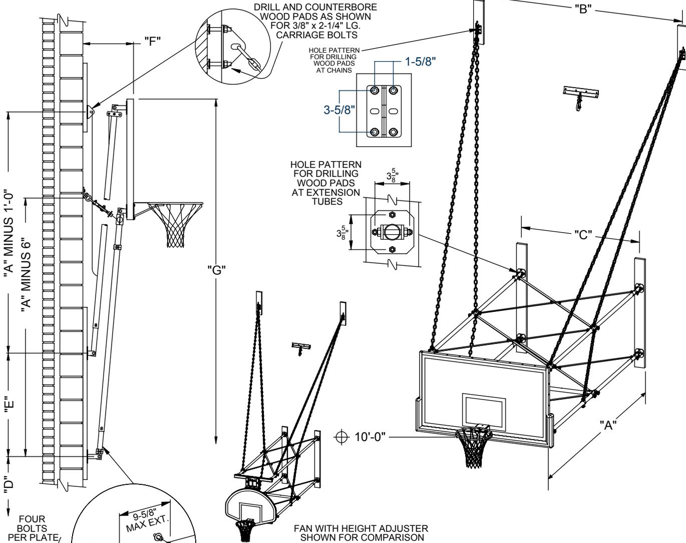
TELESCOPING EXTENSION TUBE FEATURE ALLOWS FOR PRECISE PLUMBING OF BACKBOARD. AFTER FINAL ADJUSTMENTS, DRILL 3/8"  $\phi$  HOLE THRU INNER TUBE AND SECURE WITH HAMMER HIT RIVET.
