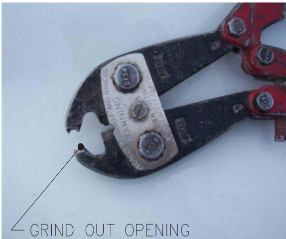
Cable cutter modified for closing "S" hooks
