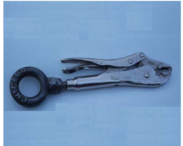
Vise-Grips modified for a variety of special uses including closing "S" hooks
