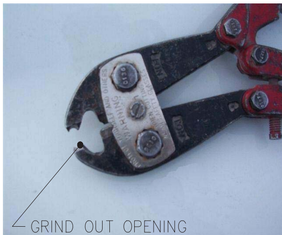
Cable cutter modified for closing "S" hooks
