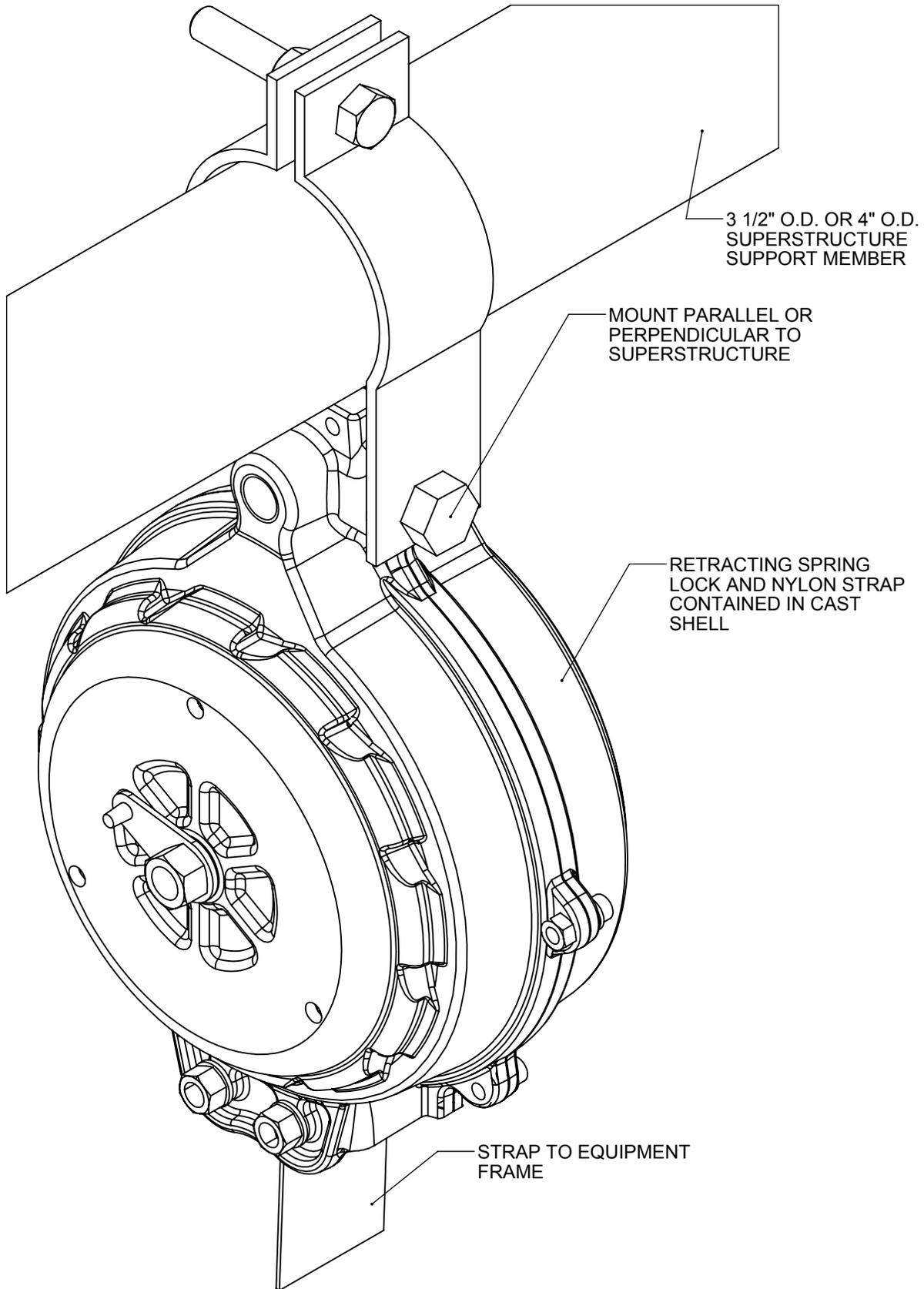
\_\_\_\_\_ - 797 LOCKING SAFETY STRAP FOR OVERHEAD EQUIPMENT
