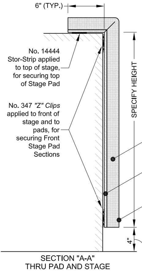
MAXIMUM ALLOWABLE DIMENSION TO MINIMIZE THE POSSIBILITY OF BODY CONTACT WITH THE WALL (Per ASTM Standard Specification F2440)
