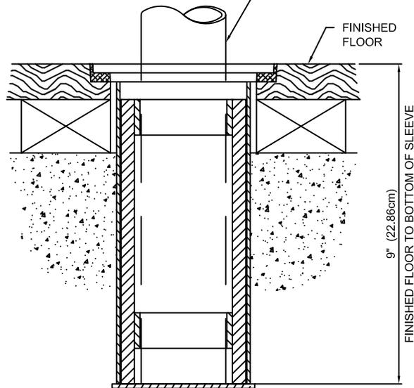
SECTION SHOWING SLEEVE ADAPTER IN PLACE IN STANDARD 3-1/2" INSIDE DIAMETER FLOOR SLEEVE
