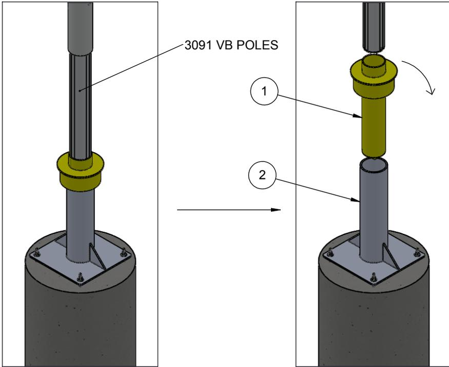
REMOVABLE SAND CATCHER PREVENTS SAND, WATER, & DEBRIS FROM ENTERING GROUND SLEEVE
