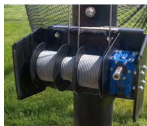
Winch and cable designed for single-person operation
