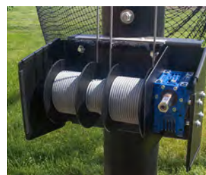
Winch and cable designed for single-person operation
