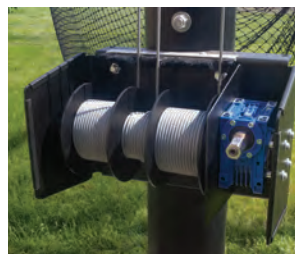
Winch and cable designed for single-person operation
