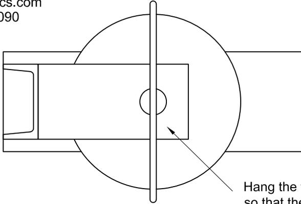
Hang the weight on the gauge so that the handle is over the hole in the top arm.
