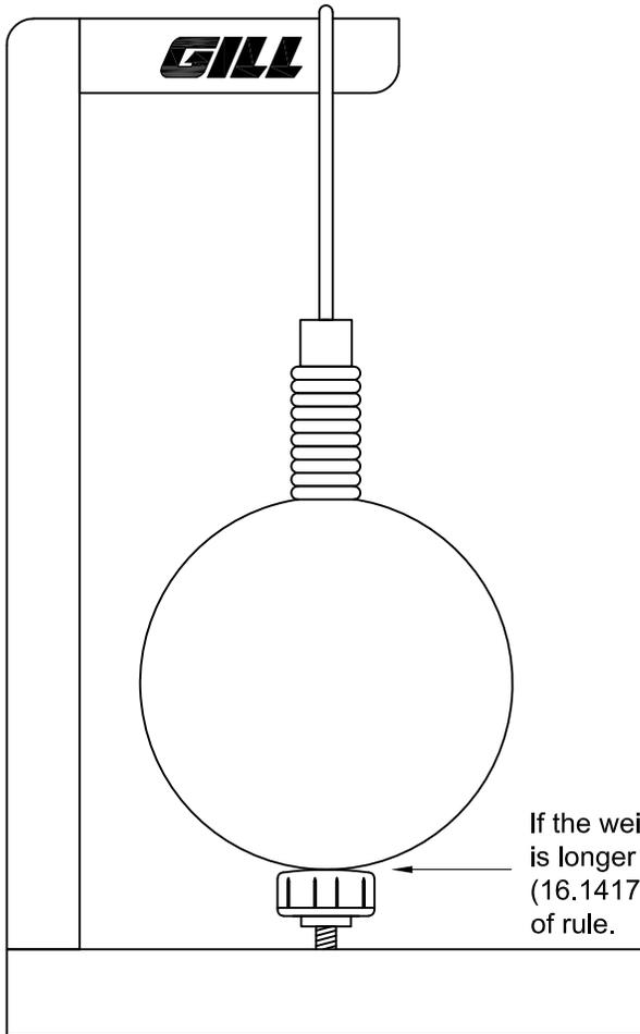
If the weight hits the knob, it is longer than 41 cm (16.1417") and therefore out of rule.
