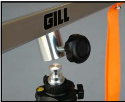
Place the adapter (and cross bar) on to the top of the tripod.
