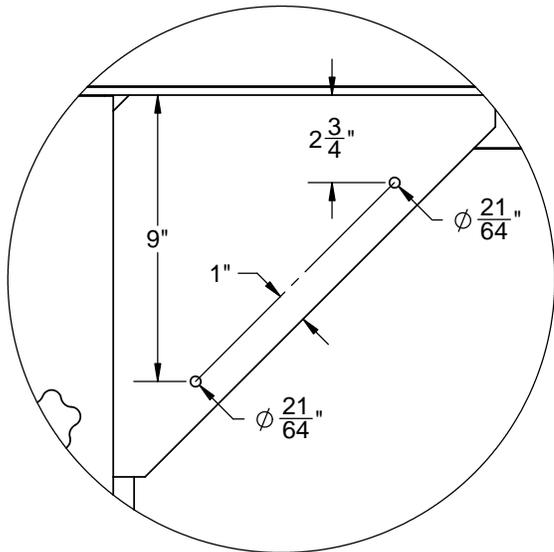
Second, mount the aluminum barrier seal to the gussets.
