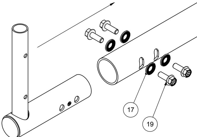
9. Slide the upright onto the elbow joint and secure it with bolts, washers, and nylock nuts.
