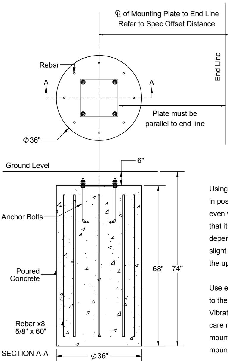
Locate the position of the goal post according to plans and specs. Excavate a hole which is at least 36" across and 74" deep. Set a form for a concrete foundation. A 36" diameter cardboard tube or corrugated metal pipe is recommended. The top of the form should be 6" below finished grade (for artificial infill turf fields, use top of infill material as finished grade elevation). Locate the formwork so that the mounting plate and anchors will be centered within the form.
