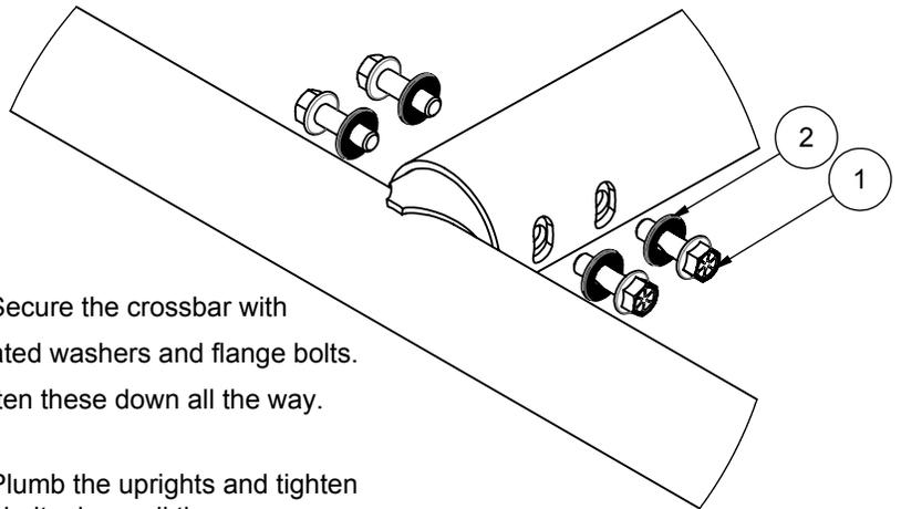
13. Secure the crossbar with serrated washers and flange bolts. Tighten these down all the way.
