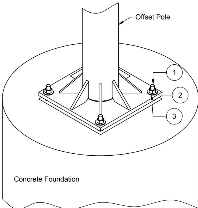
1. **After the concrete foundation has fully cured**, bolt the offset pole to the foundations using 3/4"-10 SS hex nuts (M2776) and washers (M2541) as shown.
