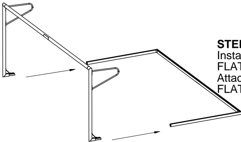
**STEP 5:** Insert front frame into base frame. Install hardware as shown in Detail "G". FLAT58702 can be adjusted as needed. Attach hardware through holes in FLAT48721E0
