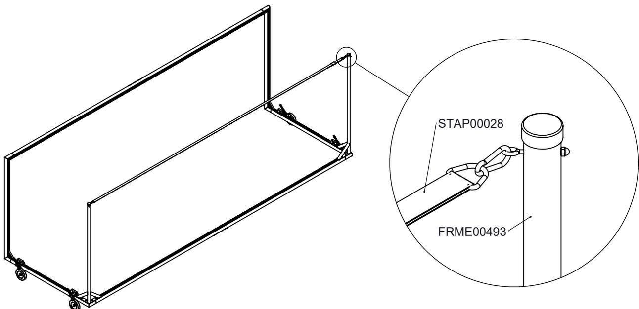
**STEP 9:** Attach the net using the provided net clips (FITG84160).
