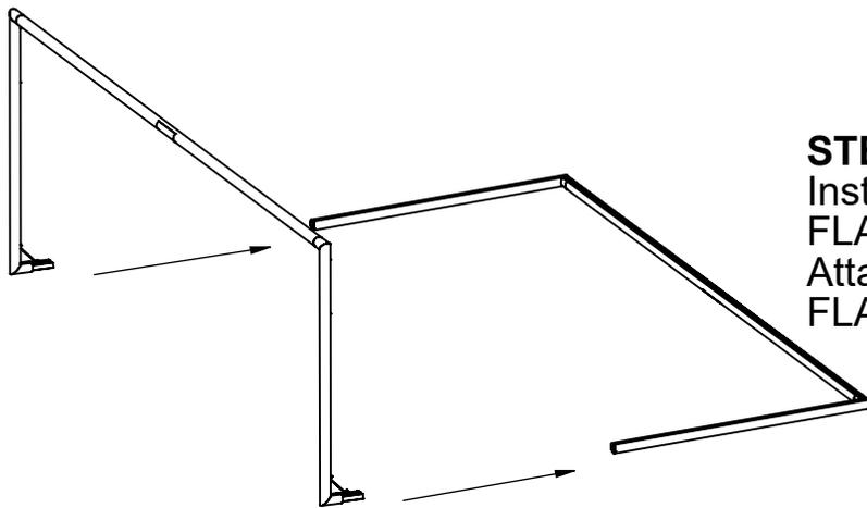
**STEP 5:** Insert front frame into base frame. Install hardware as shown in Detail "F". FLAT58702 can be adjusted as needed. Attach hardware through holes in FLAT48721E0
