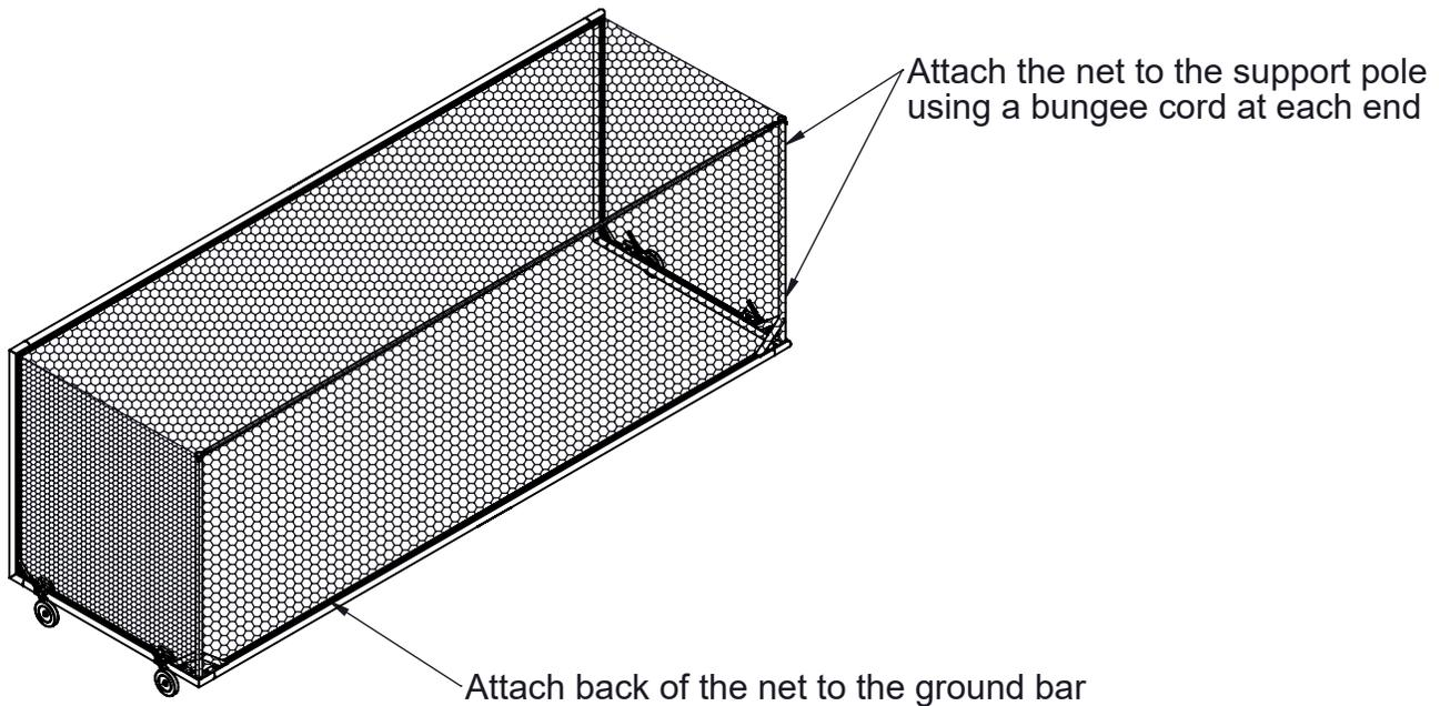
**STEP 10:** Check and tighten all hardware connections. Confirm wheels rotate and engage. Tighten net strap as needed.
