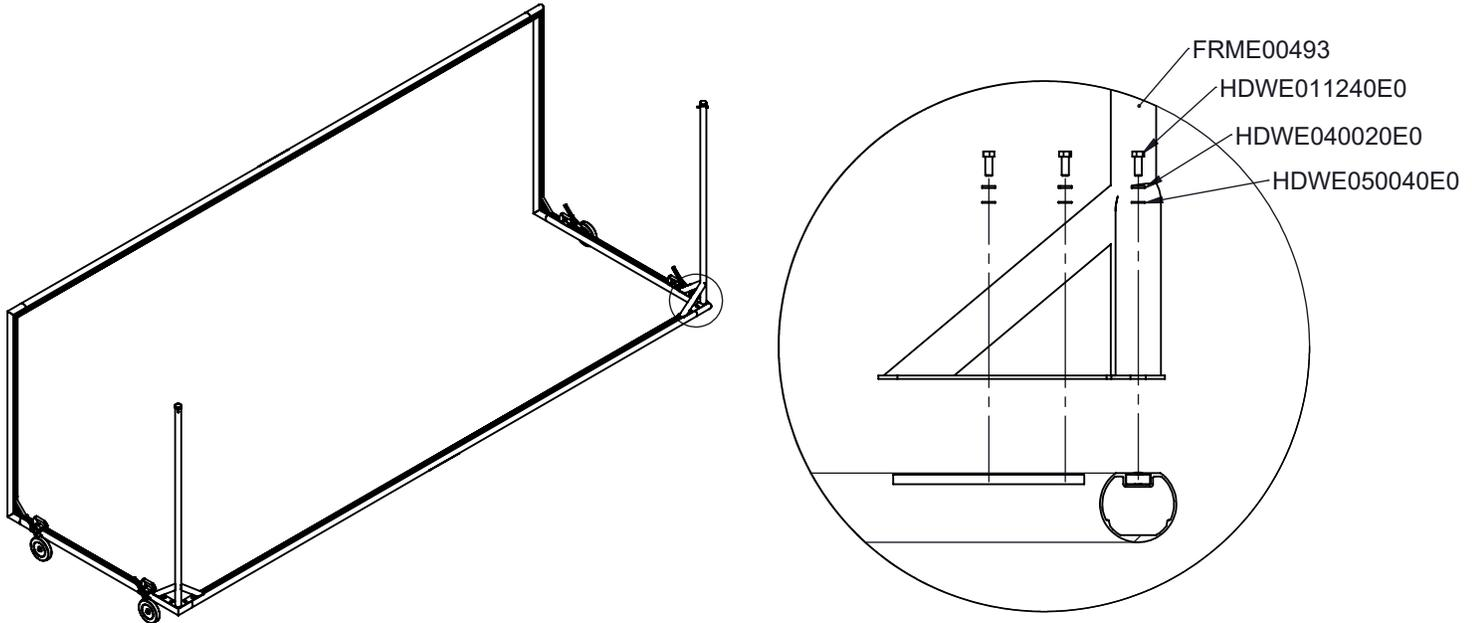
Connect the poles with the net support strap (STAP00028). Tension on the strap will keep support poles straight.
