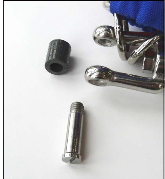
2. Slide the rings of the harness into the swivel yoke. While re-installing the threaded pin, place the spacer between the yokes and run the pin through it. Tighten down the threaded pin.
