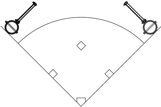
ONE SET OF SLOTS MUST BE PARALLEL AND ONE MUST BE PERPENDICULAR TO FOUL LINE. UPPER POLE SECTIONS CAN BE MOUNTED IN 90 DEGREE INTERVALS (24', 32', & 40')
