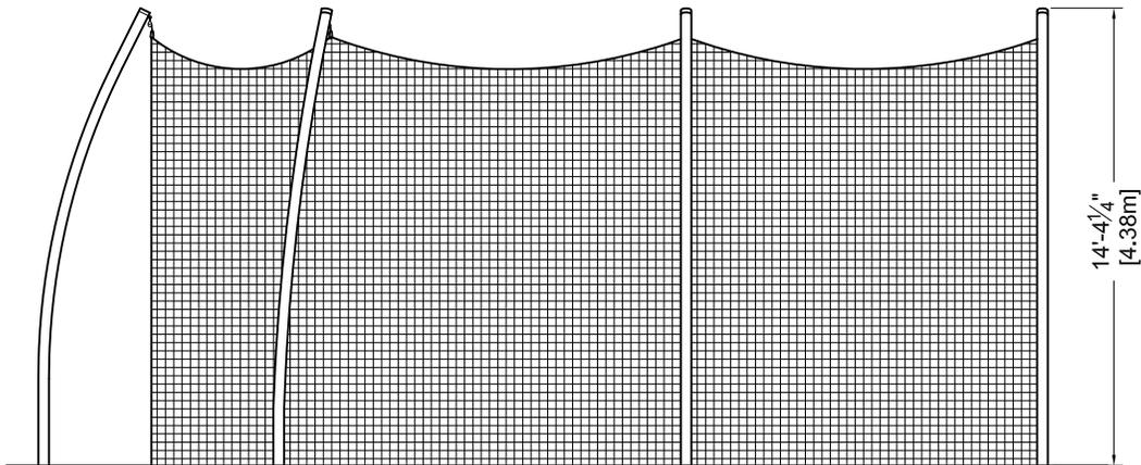
The 9020 Heavy Duty High School Discus Cage, consists of seven, 14' tall, rolled aluminum net poles with ground sleeves, a vinyl coated net support cable to reduce net sag, and a weather treated nylon net. Hinged net arms, at ground level, hold the net in place at the front of the cage. The poles are 4" OD, 0.218 wall, 6063-T6 aluminum tube. Each pole stands in a 36" deep ground sleeve. The net is 180 lb. test nylon which has been weather treated for extended service life.
