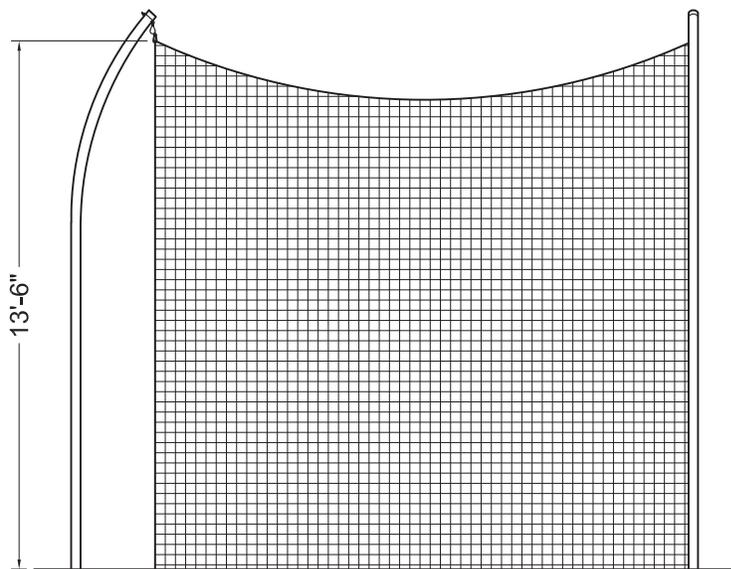
The 8050 Shot Put Cage, consists of four, 14' tall, rolled aluminum net poles with ground sleeves, a vinyl coated net support cable to reduce net sag, and a weather treated nylon net. Hinged net arms, at ground level, hold the net in place at the front of the cage and anchored eyebolts at the back. The poles are 2 7/8" OD, 0.203" wall, 6063-T6 aluminum tube. Each pole stands in a 30" deep ground sleeve. The net is 180 lb. test nylon which has been weather treated for extended service life.
