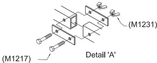
**NOTE:** Front extension stringers run underneath front panel planks with their ends even with the back edge of the front plank.
