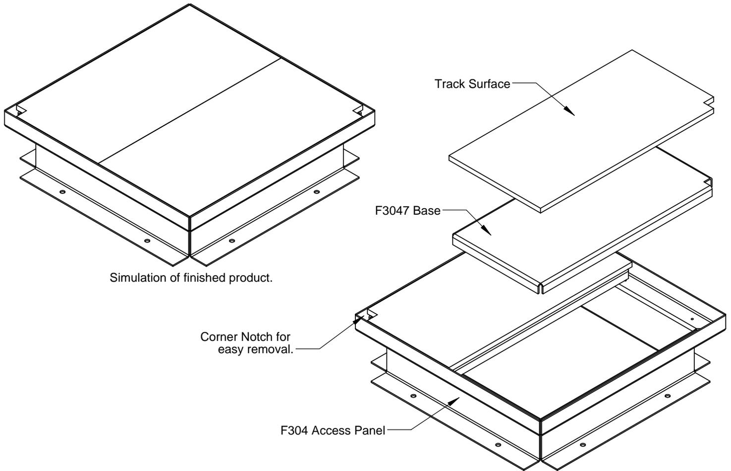
The F3047 Solid Plug for the F304 Access Panel serves as a base to pour or roll out track surface onto. This is great for fields where the football goal is mounted in the D-zone of a track. The base is made of .125" folded aluminum with a notched corner for easy removal. The base comes in two pieces and the customer is responsible for attaching the track surface.
