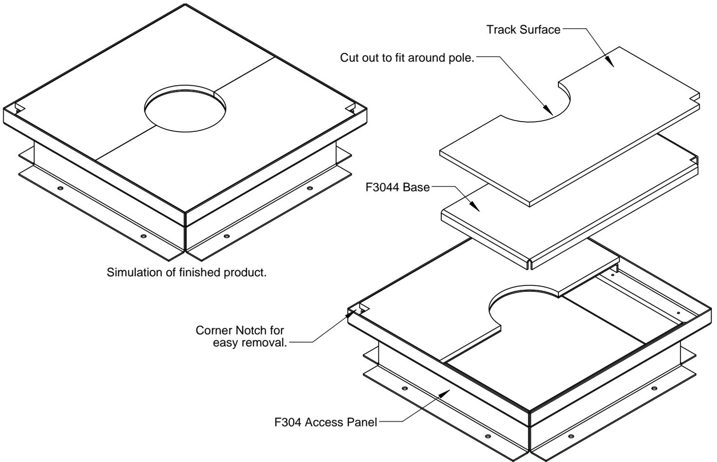
The F3044 Pole Plug for the F304 Access Panel serves as a base to pour or roll out track surface onto. This is great for fields where the football goal is mounted in the D-zone of a track. The base is made of .125" folded aluminum with a notched corner for easy removal. The base comes in two pieces and the customer is responsible for attaching the track surface.
