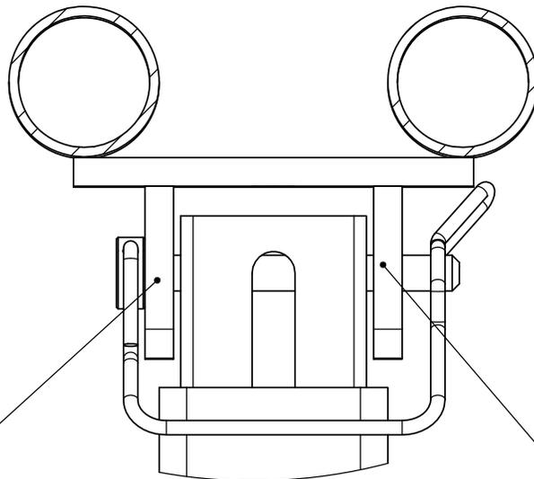
ONE END OF THE RAIL HAS TWO FLATS WELDED ON (SHOWN ABOVE). THESE FLATS WILL STRADDLE THE UNISTRUT.
