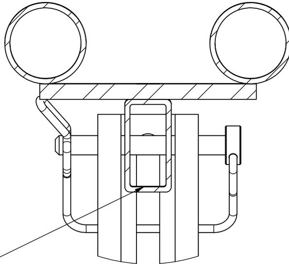
ONE END OF THE RAIL HAS A RECTANGULAR TUBE WELDED ON (SHOWN ABOVE). THIS TUBE WILL SLIDE INTO THE OPENING OF THE UNISTRUT.
