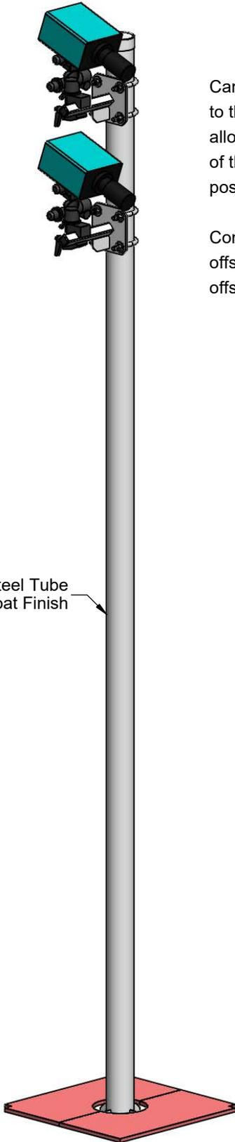
Camera offsets are mounted to the upright with u-bolts to allow for infinite adjustment of the camera height and position.
