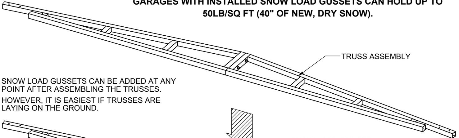
SNOW LOAD GUSSETS CAN BE ADDED AT ANY POINT AFTER ASSEMBLING THE TRUSSES. HOWEVER, IT IS EASIEST IF TRUSSES ARE LAYING ON THE GROUND.
