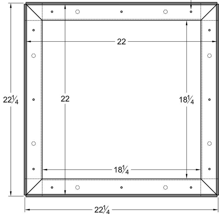
$\text{Ø}\frac{3}{16}$ " hole for wood furring strip attachment if needed
