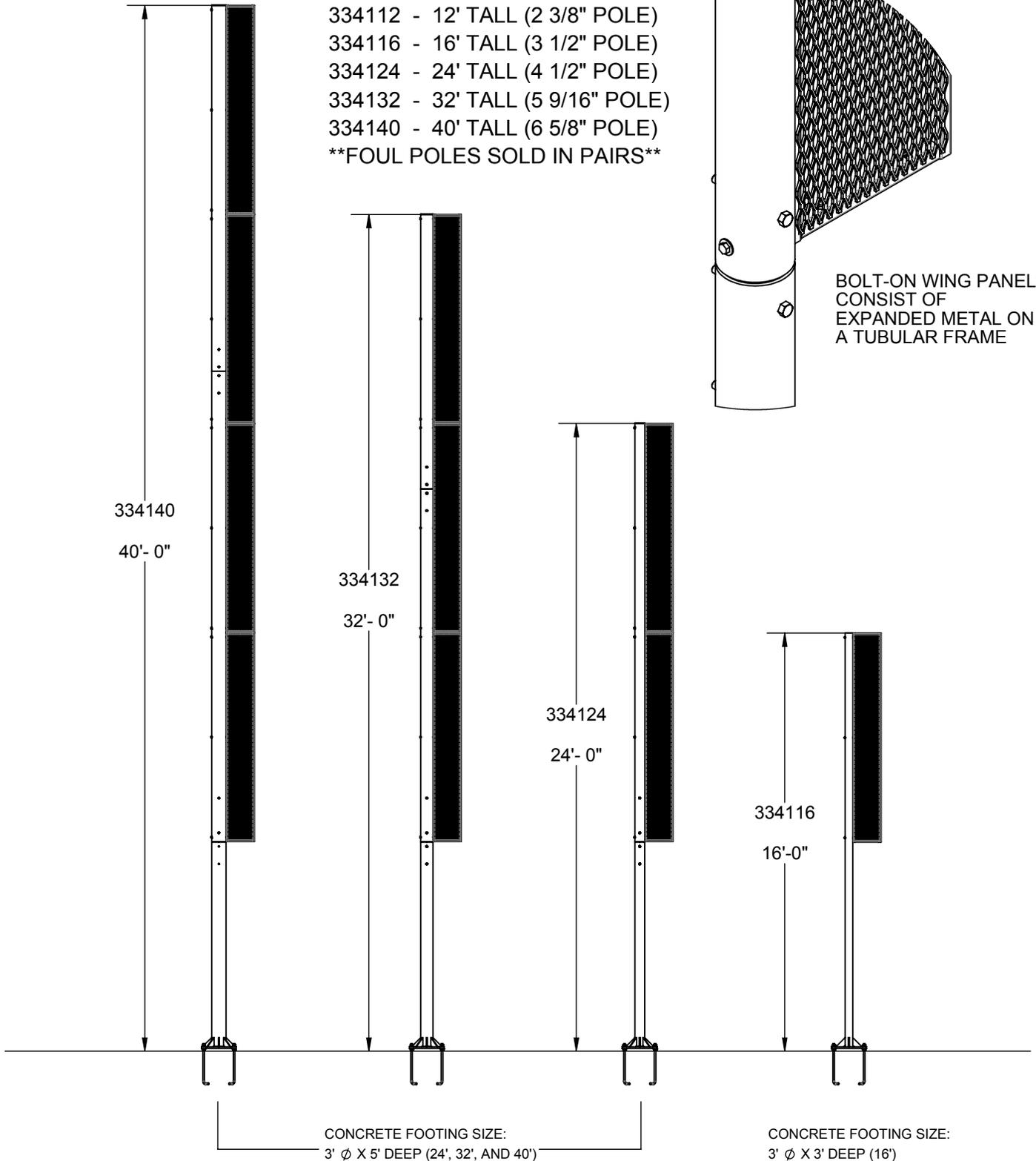
THIS IS THE MINIMUM RECOMMENDED FOOTING SIZE. INCREASE SIZE OF FOOTING AS REQUIRED ACCORDING TO LOCAL SOIL CONDITIONS, AND TO MEET LOCAL BUILDING CODES REGARDING MINIMUM WIND SPEEDS.
