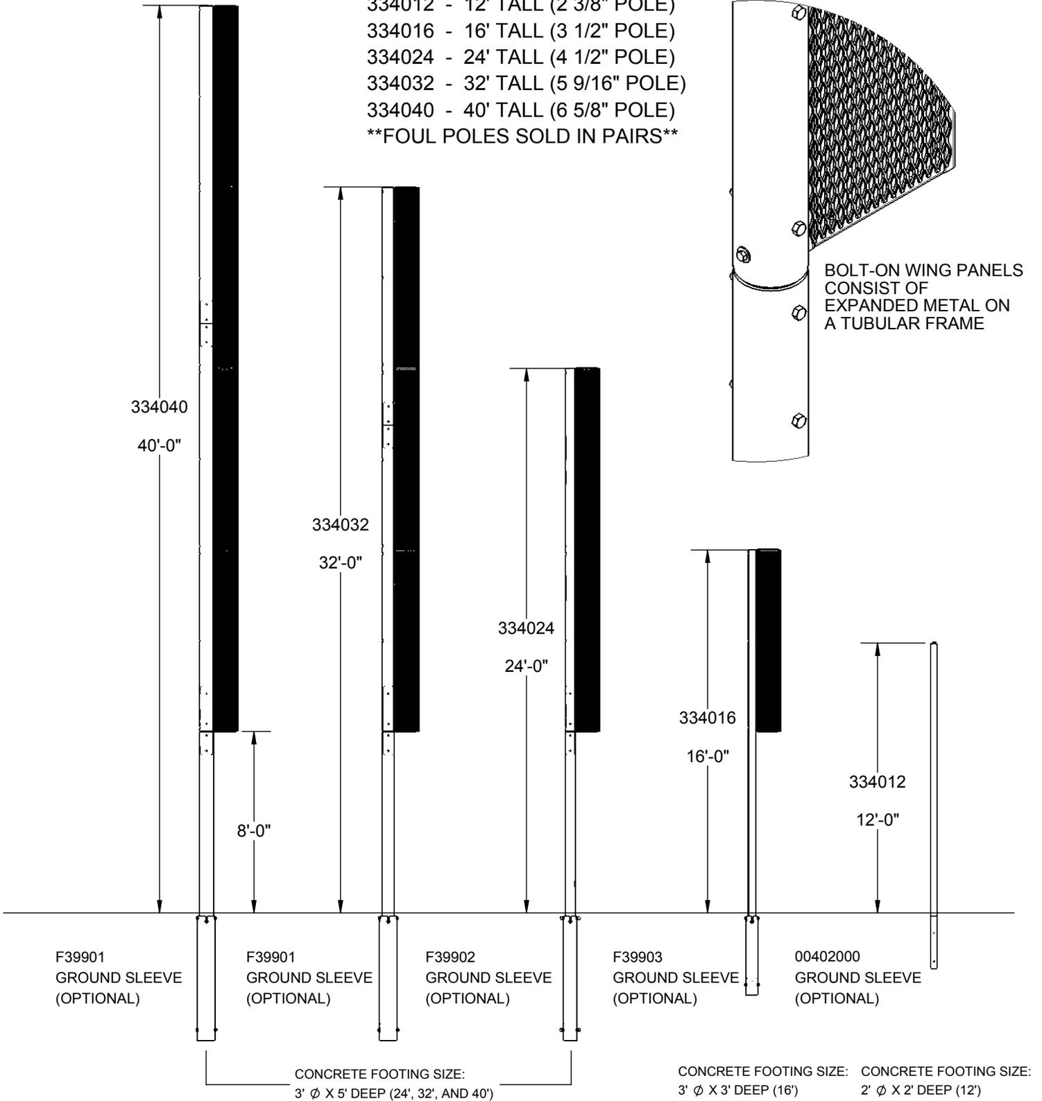
THIS IS THE MINIMUM RECOMMENDED FOOTING SIZE. INCREASE SIZE OF FOOTING AS REQUIRED ACCORDING TO LOCAL SOIL CONDITIONS, AND TO MEET LOCAL BUILDING CODES REGARDING MINIMUM WIND SPEEDS.
