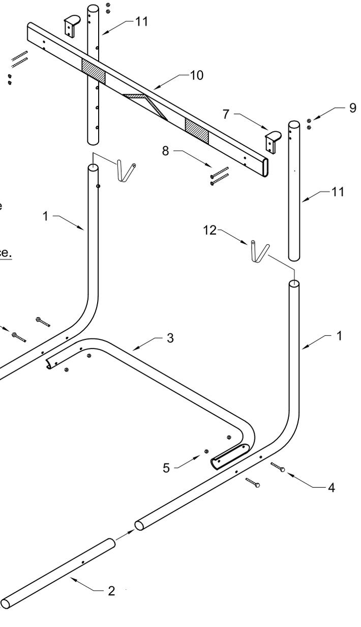
Legs are boxed with leg weights installed and held in place with orange plugs. To remove plastic plugs, insert a bolt (#4) into the opposite side and push the plug out.
