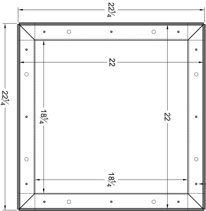
Ø3/16" hole for wood furring strip attachment if needed
