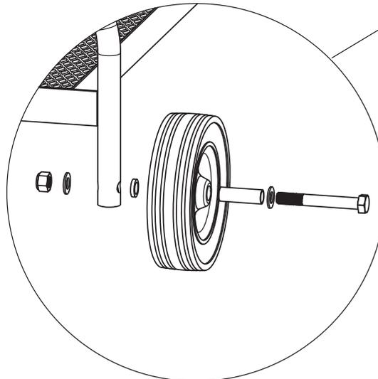
Fasten wheels to the rear A-Frame with one bolt, three washers, a nut, and hub reducer per wheel.
