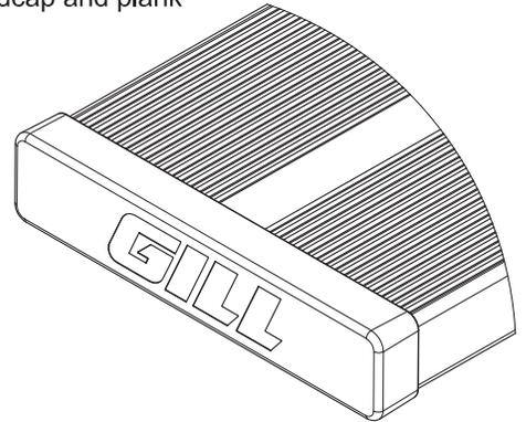
Install endcap onto end of plank. Secure in place with two self drilling screws. Repeat for the other end of plank.
