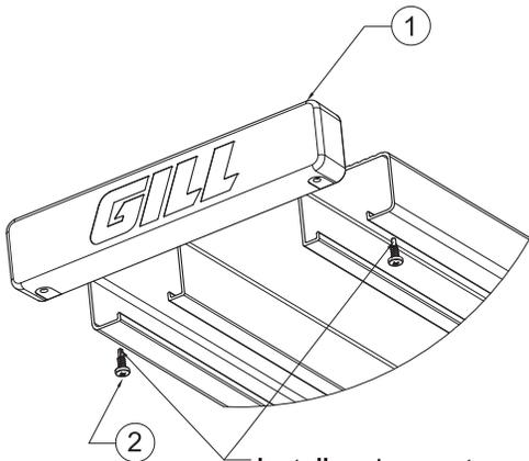
Appearance of assembled endcap and plank
