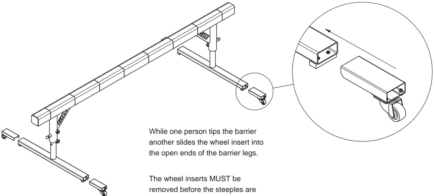
While one person tips the barrier another slides the wheel insert into the open ends of the barrier legs.
