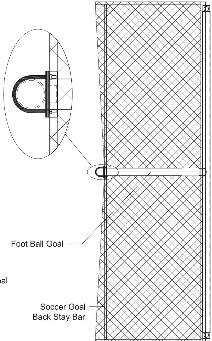
NOTE: If back stay bar is wider than 2" the spacer nut may need to be used to tighten the clamp bar and the other hex nut used to tighten the goal trap bracket.
